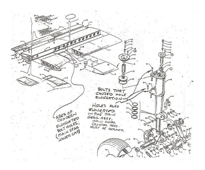
Piper PA17, Worn Landing Gear Mount Holes, ATA 3211
